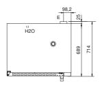
E: Electric connection D: Drain for water H2O: Water inlet 3/4"
